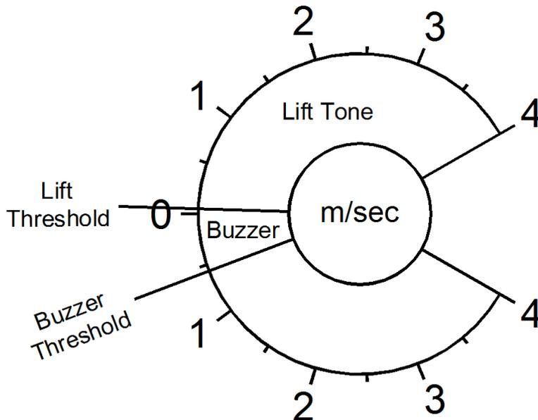
The buzzer tone frequency increases as my sink rate reduces until I get an actual climb and the lift tone takes over.
