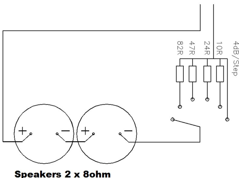
The resistors shown give settings of 4dB of volume per step and I use a TT
