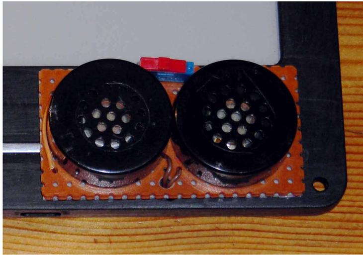
On this Kobo the speakers are mounted on a piece of stripboard fixed with double sided foam tape. There is also a small pcb slide switch visible at the top to switch the audio on and off.
