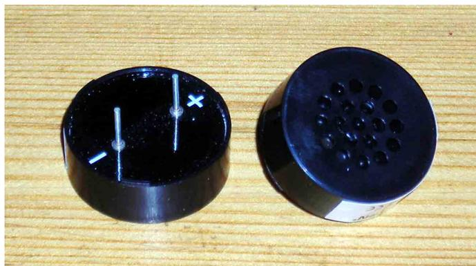
These are quite expensive but cheaper versions are available such as the Ekulit AL-23P. They are both 23mm in diameter and inside the housing is a 19mm diameter speaker.
