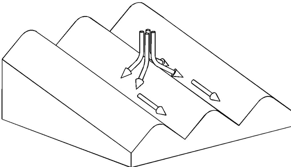
If we are low over a spine and encounter sink we are likely to drop down into the adjacent clough in the sinking air. Not nice!
