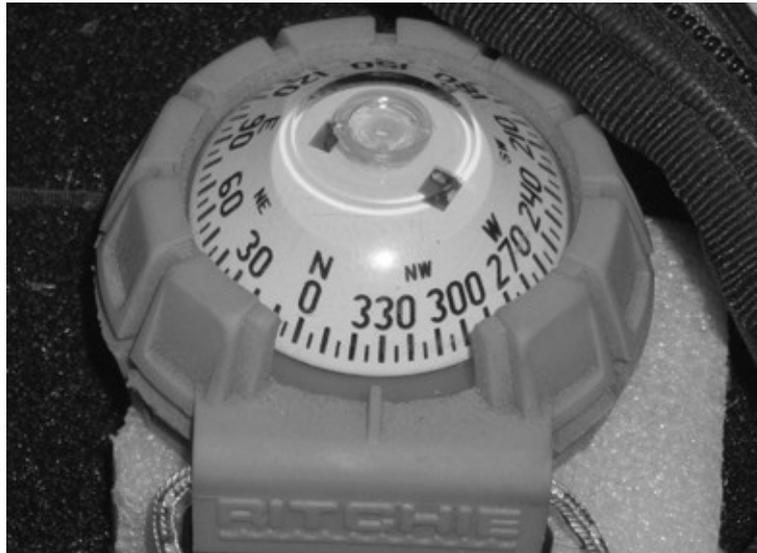
We must be careful where we position our compass on our flight deck. Any nearby magnetic material will cause it to misread. Other instruments and radios are likely to have magnetic material in them. Some batteries can be magnetic.
